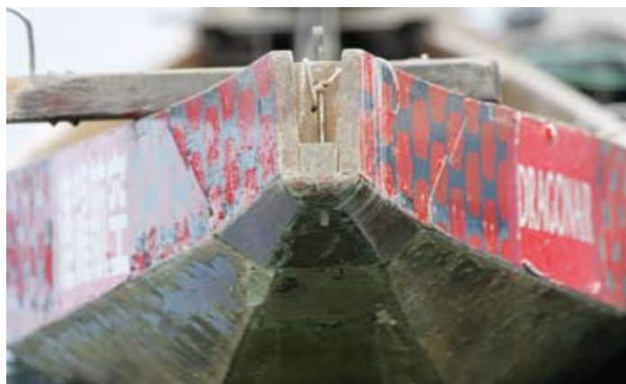
Picture 2: With this boat the keel plank itself has no conical shape therefore the shape is made with the inner bottom planks (see Picture 4)
