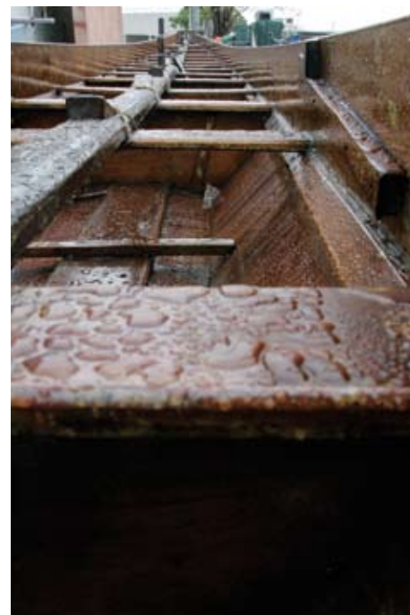
Picture 8: The inside of a boat clearly shows the supporting wedge, fixtures of seats and spine as well as a bulk head with small water-through-let-holes can be seen. This boat also carries additional holding bars for the outer bottom planks. The bars are fixed on the keel plank
