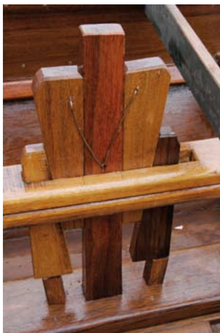
Picture 7: The mechanism to stiffen the hull, located in the boat's middle. The pressure is applied directly to the keel plank
